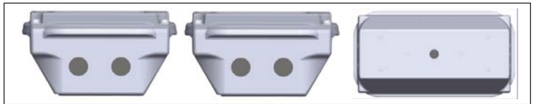
Option "H" 2 Entries One Side, 2 Entries Opposite Side and 1 Entry in the Rear Add H to the end of the order code
